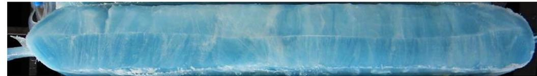
The 10L bag in the plate freezer shows a significant homogeneous coloring image as the 10L bag which was frozen in the static freezer.
